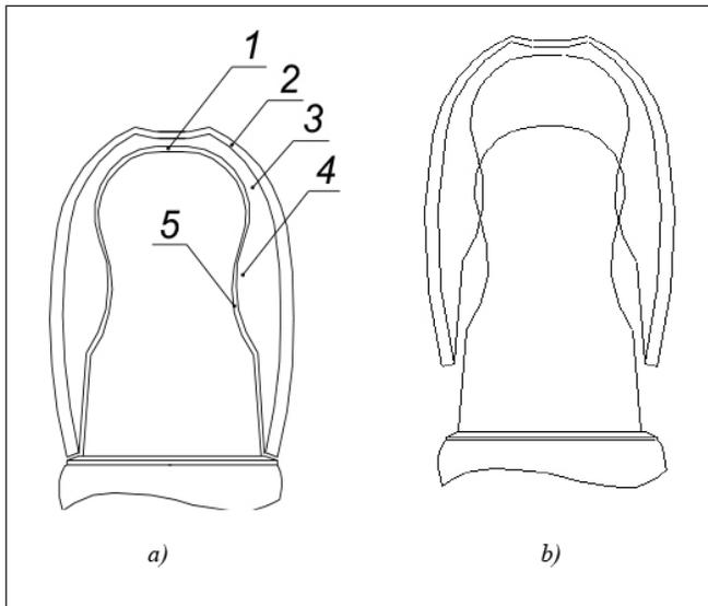
**Figure 1.** Scheme of the device of the telescopic connection: a) - the working position of the "lock"; b) - the position of elastic deformation.
