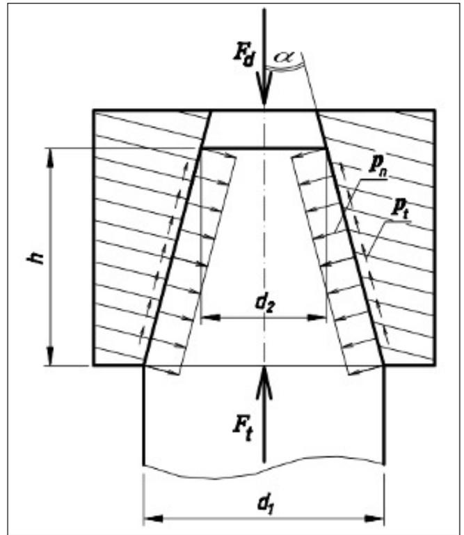
**Figure 2.** Scheme of conical connection
