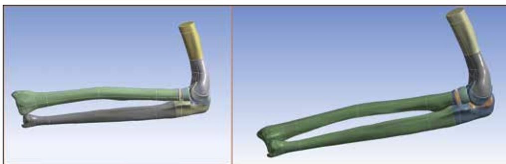
Fig. 1. Two geometric models of elbow joint with bipolar RH endoprosthesis in a neutral semipronation and 90° elbow flexion.
