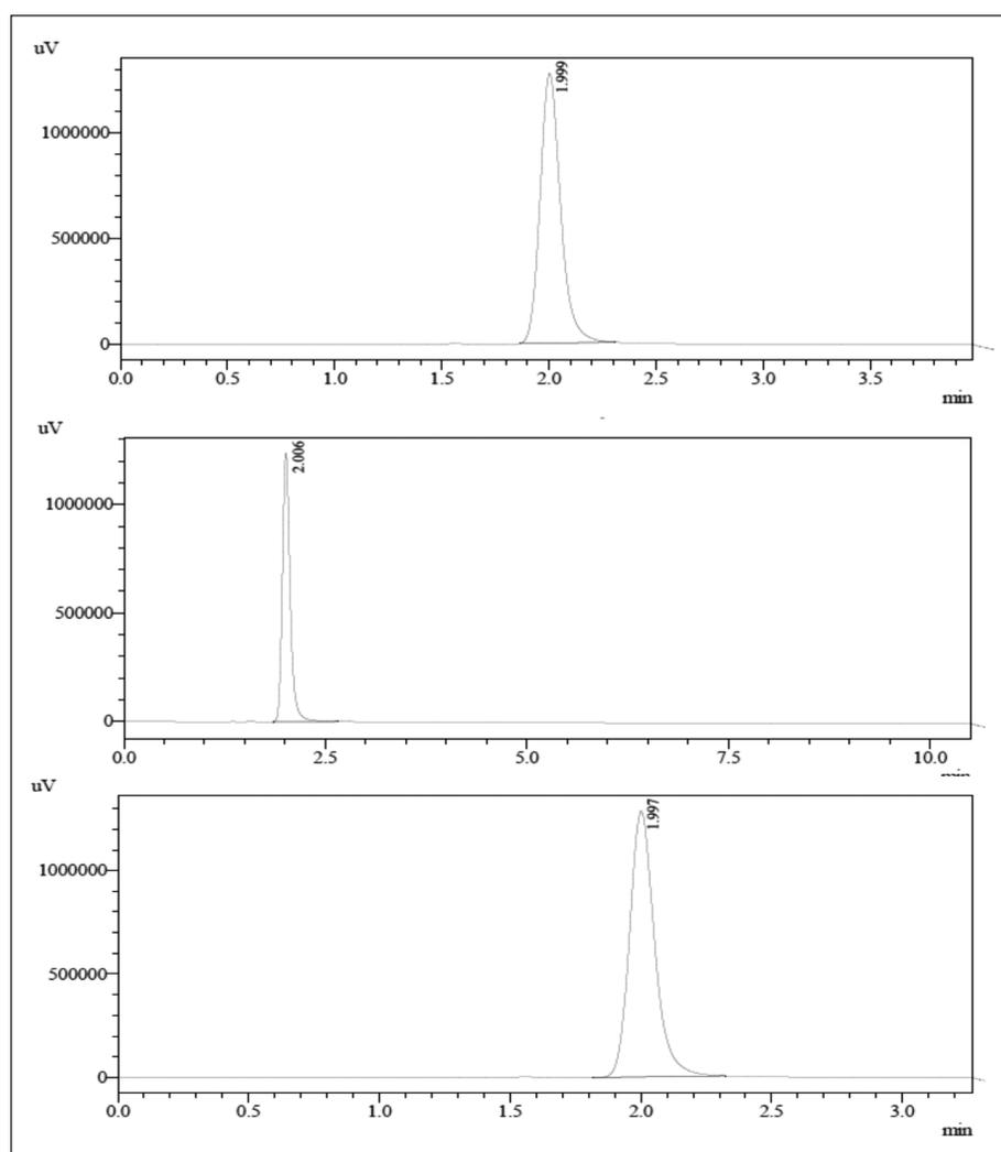
**Fig. 5.** Chromatographs of standard solution
