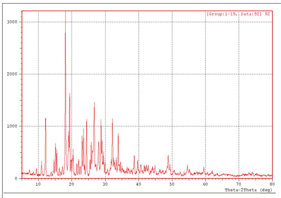
**Fig. 9.** X-ray Diffraction Pattern for Ceftriaxone Raw Powder
