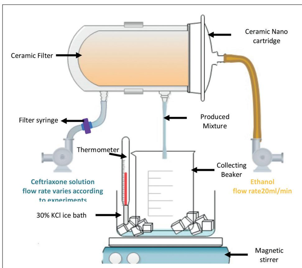
**Fig. 3.** Continuous crystallization by ceramic filter
