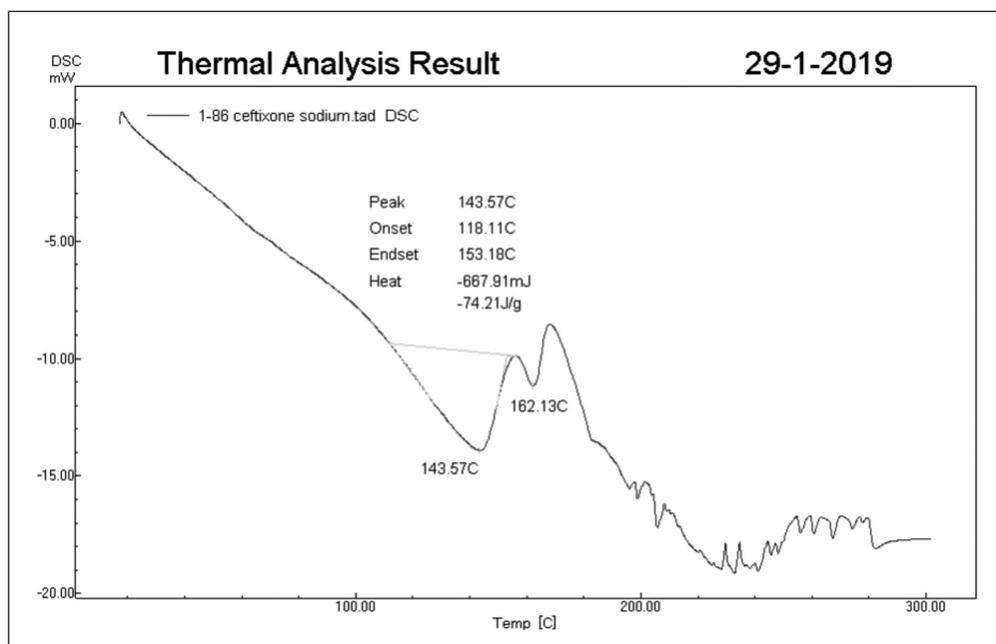
**Fig. 18.** Thermogram of Ceftriaxone Raw Powder
