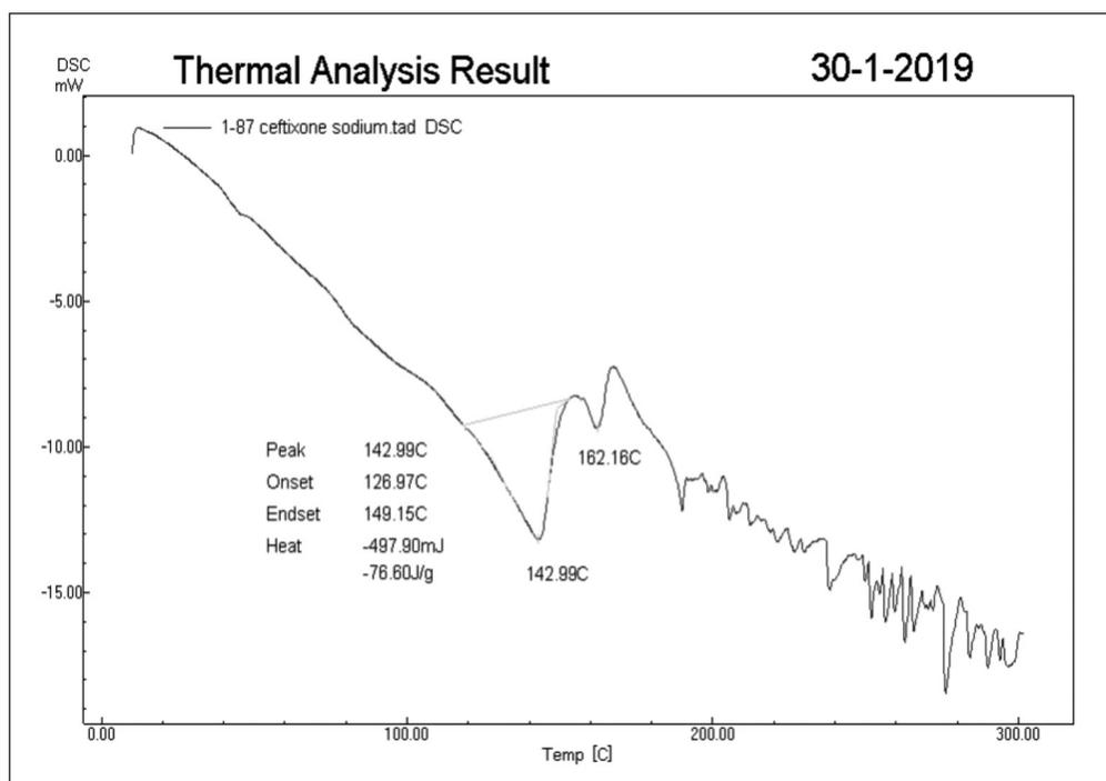
**Fig. 19.** DSC Thermogram F2Filter
