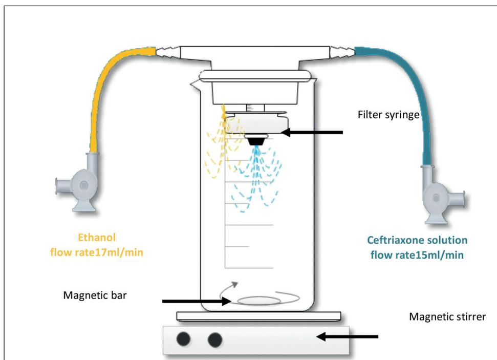
**Fig. 2.** Schematic illustrate the simple mixing method
