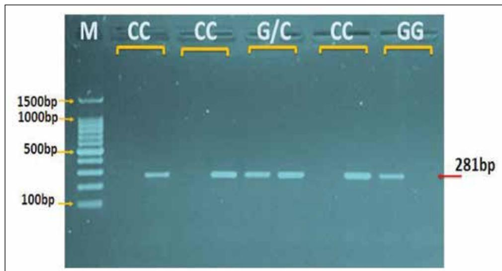
**Fig. 1.** Agarose gel electrophoresis image showed the ARMS-PCR product analysis of rs1800795 (C/G) gene polymorphism. Where M: marker (1500-100bp). The presence of A or G allele was observed at 281bp product size. The (GG) wild type homozygote was present in G allele only, the (CC) mutant type homozygote showed in C allele only, whereas the (G/C) heterozygote showed in both G and C allele.
