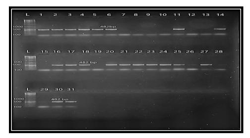
**Fig. 1.** In a Monoplex PCR agarose gel, amplified products from extracted DNA of Gram-negative isolates and amplified with primers and the primer genes acc(6)-lb were amplified. The electrophoresis was performed at 70 volt for 1.30 hr with using DNA ladder size (plus 1000), lanes (1, 2, 3, 4, 5, 6,) show positive results at 482 bp.
